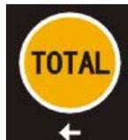
At Zero mode, load weight till stable, Press go to accumulation mode, "Total" light on, display" n 001", and then display loaded weight; unload the weight , back to zero, load the second weight again till stable. Press display"n002" then display the second loaded weight. Repeat it agin and
